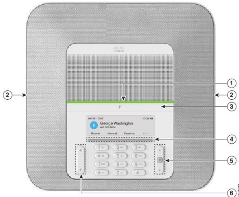
Figure 11: Cisco IP Conference Phone 8832 Buttons and Features
