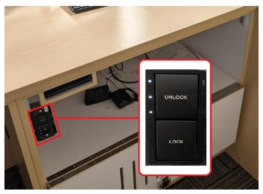
2. Inside the cabinet locate a small switch with two buttons – "Lock" and "Unlock". Press the **Unlock** button to start up the AV system.
