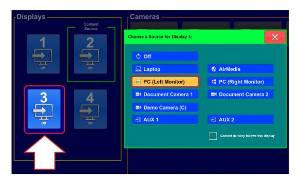
2. Then on the touchscreen panel find and press the icon for **Display #4** and then set that display to **"PC (Right Monitor)"**.
