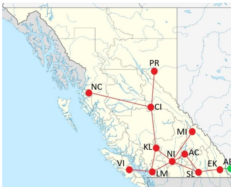
Figure 3.1: Map of British Columbia PLEXOS model showing nodes, transmission lines and intertie Alberta (AB). Original map under creative commons.
