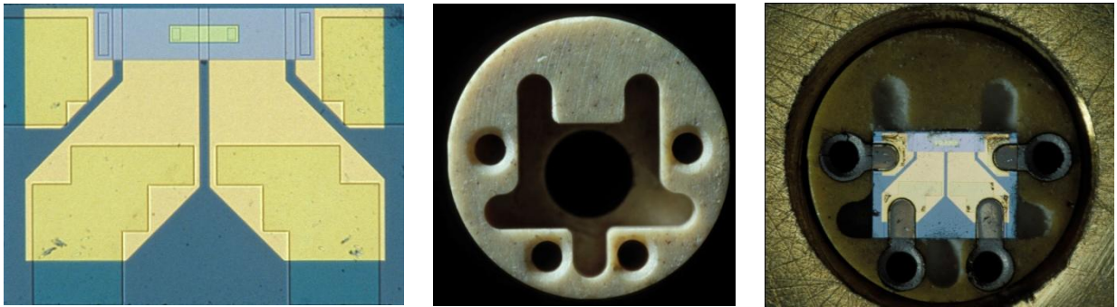
Figure 3-15- The guard-heated sensor chip, and the ceramic holder [25].
