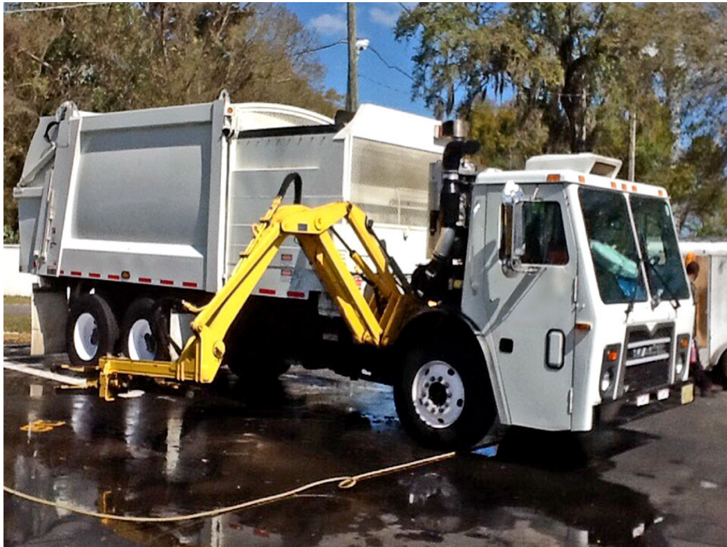
Figure 4) Heil automated side-loader refuse truck[13]
