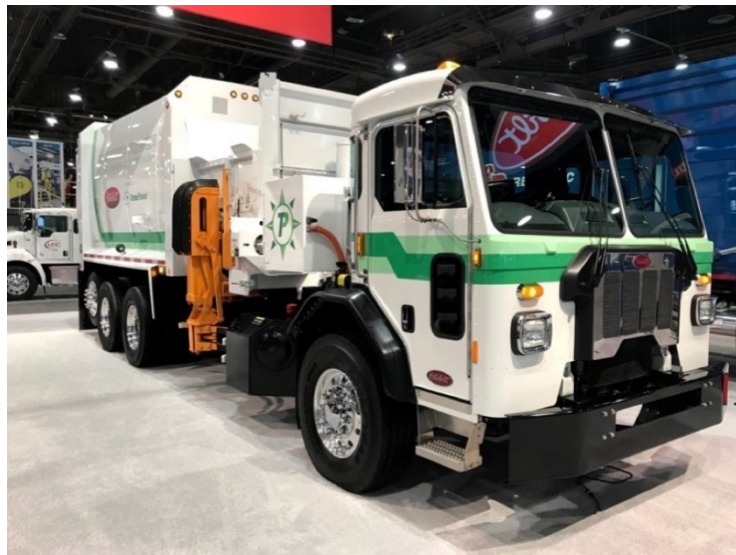
Figure 6) Peterbilt, Model 520 all-electric side-loader refuse collection truck [29]
