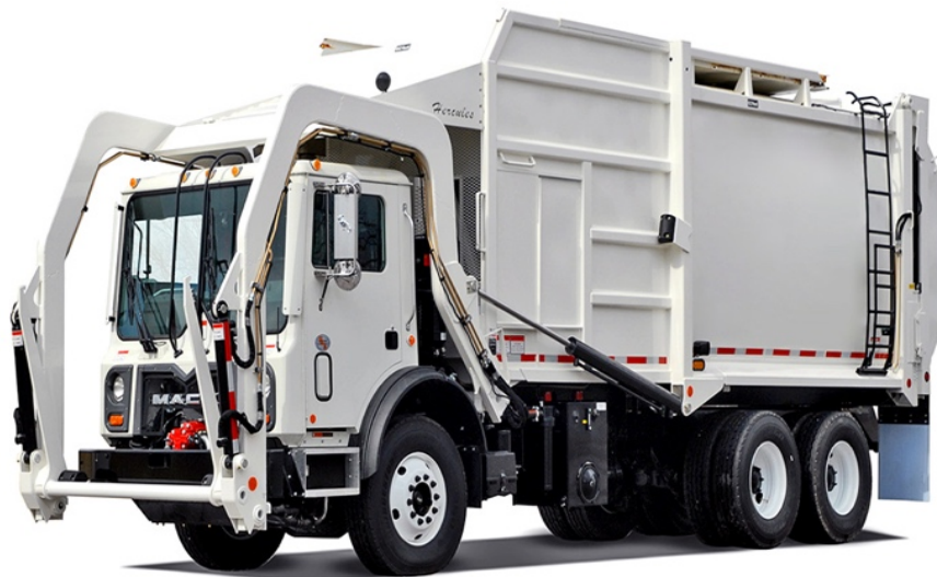
Figure 2) 2002 Mack MR690S front-loader refuse truck [13]
