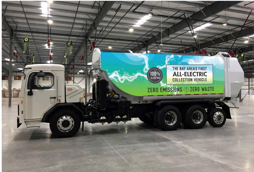
Figure 7) BYD 8R all-electric fully automated side-loader refuse collection truck [33]
