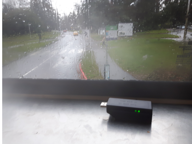
Figure 3.1: GPS Tracker Key setup to record the bus speed, elevation and GPS coordinates on a double decker
