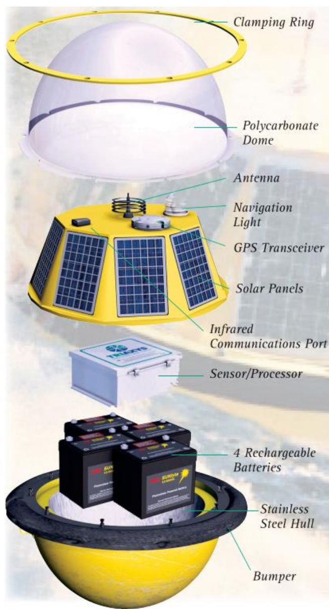
Figure 2.1 – Exploded view of the TriAXYS buoy [1]
