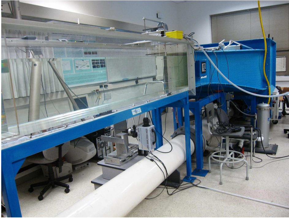
Figure 2.1 – Water tunnel which was used in the experiment
