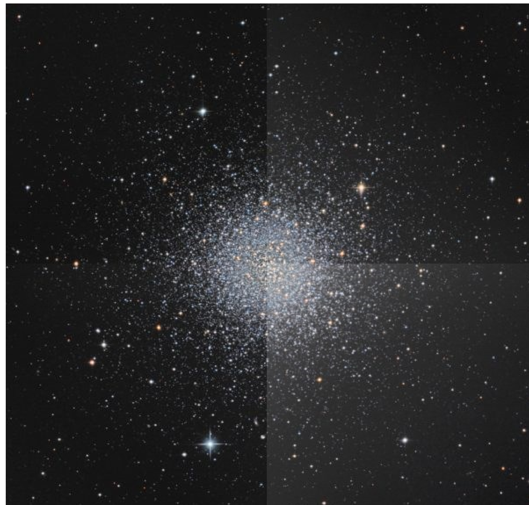
Simulated dark- and flat-corrected image before applying nonlinearity calibration
