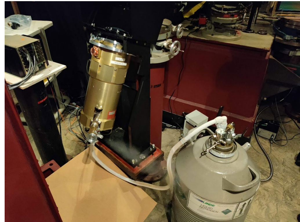
Cryostat installed on McKellar Spectrograph
