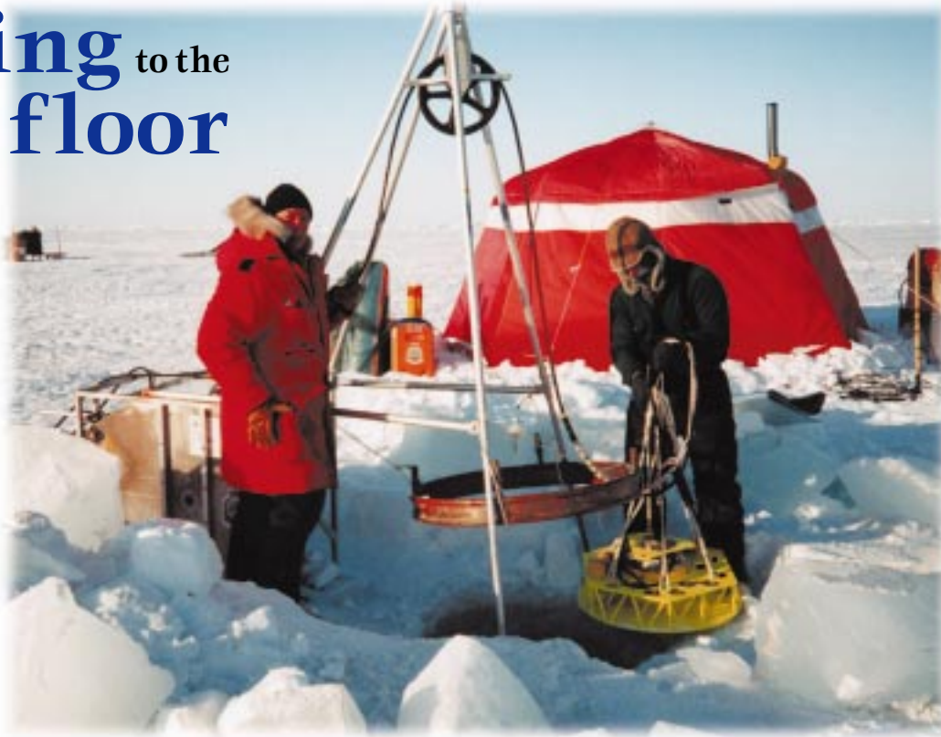
Dosso (right) and technician Jim Perkins prepare to deploy an ocean bottom seismometer to measure vibrations 500 metres beneath the Arctic sea ice.
