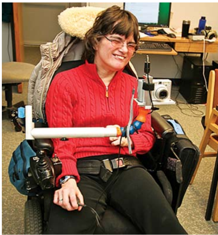
CanAssist client Val Curley, with her adjustable wheelchair camera mount. The device has a trigger system that allows her to take a picture with a squeeze of a bulb.
