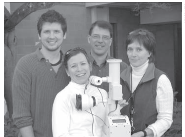
L-r: Hystad, Lightowlers, Keller and Setton. The instrument is a nephelometer, which measures particulate matter.
