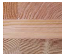
WOOD CLT STRUCTURE
