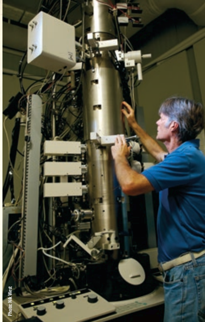
Dr. Rodney Herring works on the new scanning transmission electron holography microscope (STEHM), which is opening the door to transformative scientific research.
