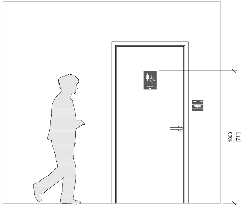
Installation of Washroom Door Signs
